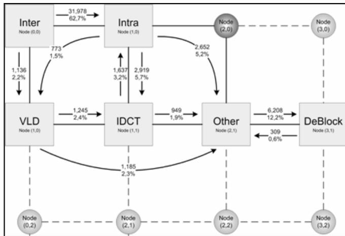
Fig. 12: Inter-component communication in the H.264 decoder.
