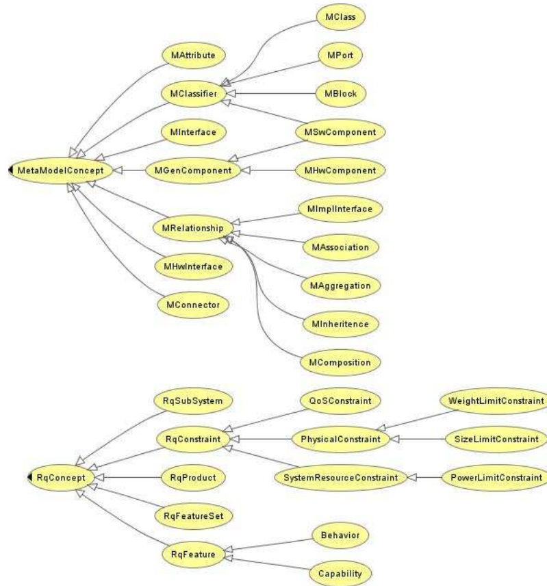
Figure 5: A snapshot of the OWL class hierarchy that forms the ODL metamodel.
